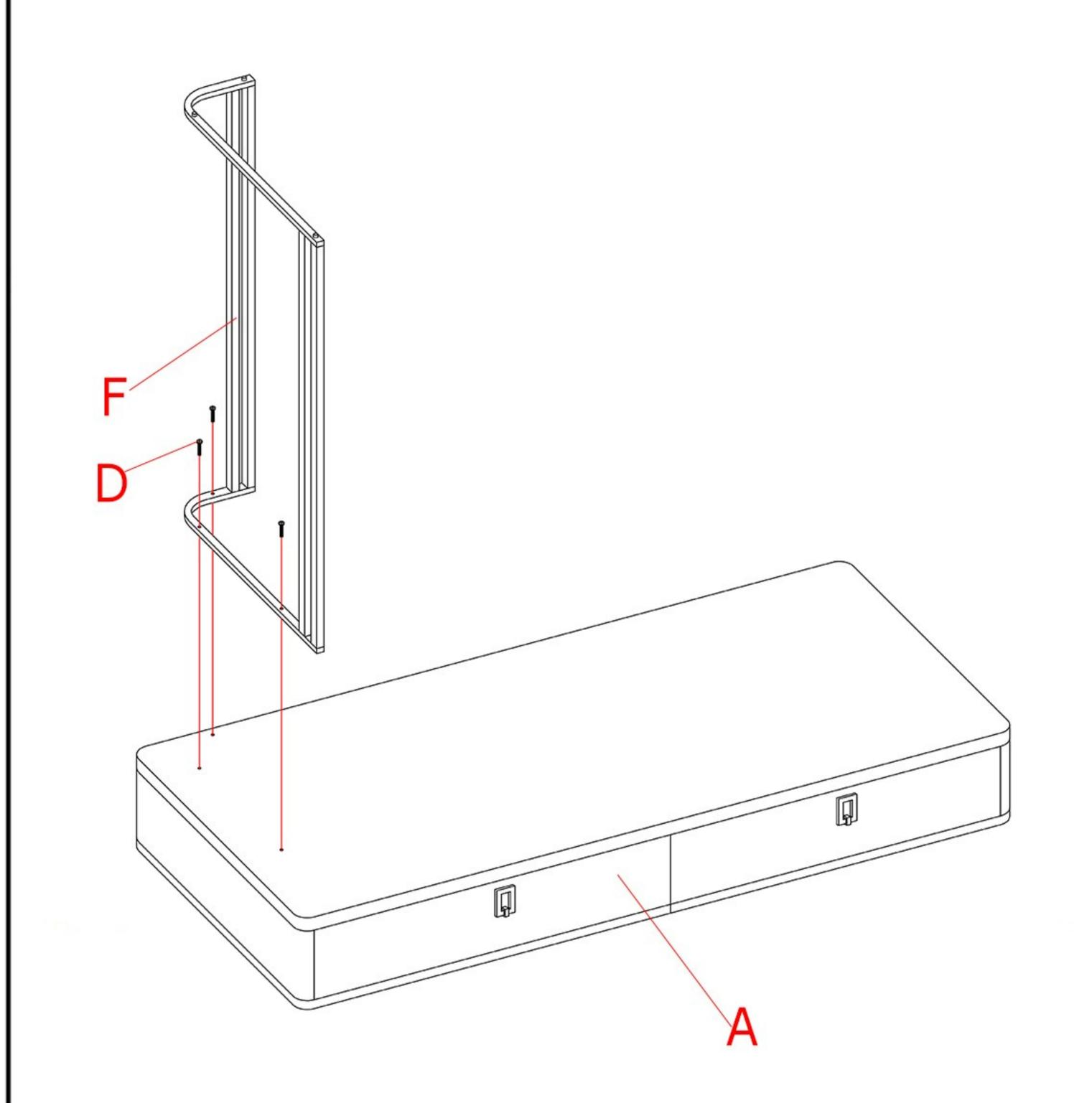
1. Put the upper table (A) upside down on clean floor cushioned by soft clothing. Align the metal frame (F) to the table hole by hole and then fix the frame to the table by driving screws (D) with a percussion drill(not included).
