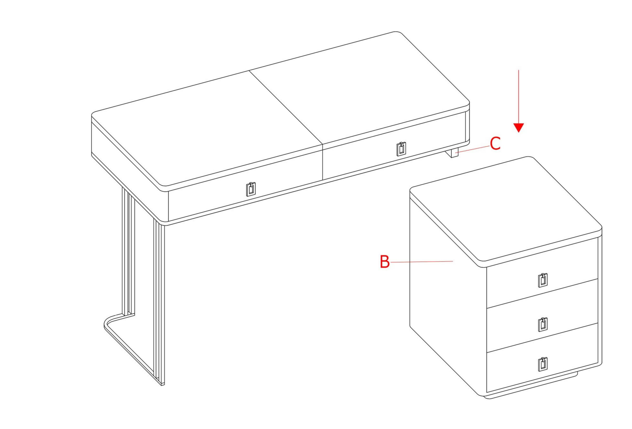
3. Stand the finished part and place the metal base (C) onto the side table (B).
