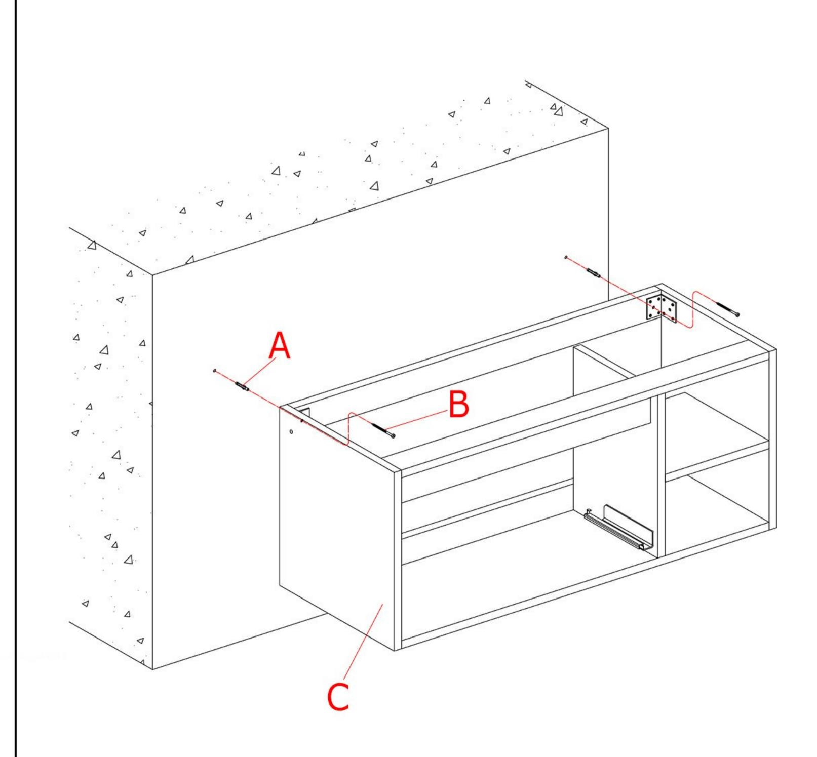
2. Put the cabinet body (C) to the wall and adjust the body to make sure that it is straight and level. According to the holes on the hinges at the corners of the body, mark to drill holes on the wall. Suit the expansion bolts (A) into the drilled holes and tighten the expansion screws (B) through the holes on the hinges into the bolts in the wall.
