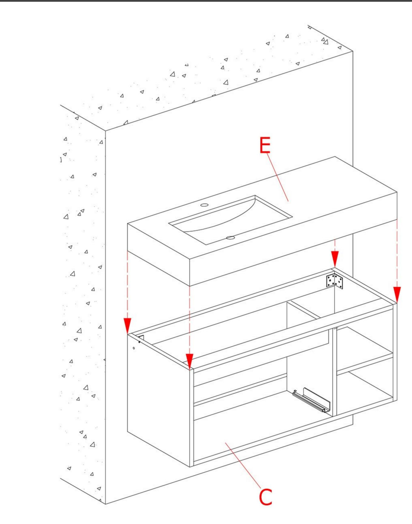
3. Put the basin (E) onto the top of the cabinet body (C).
