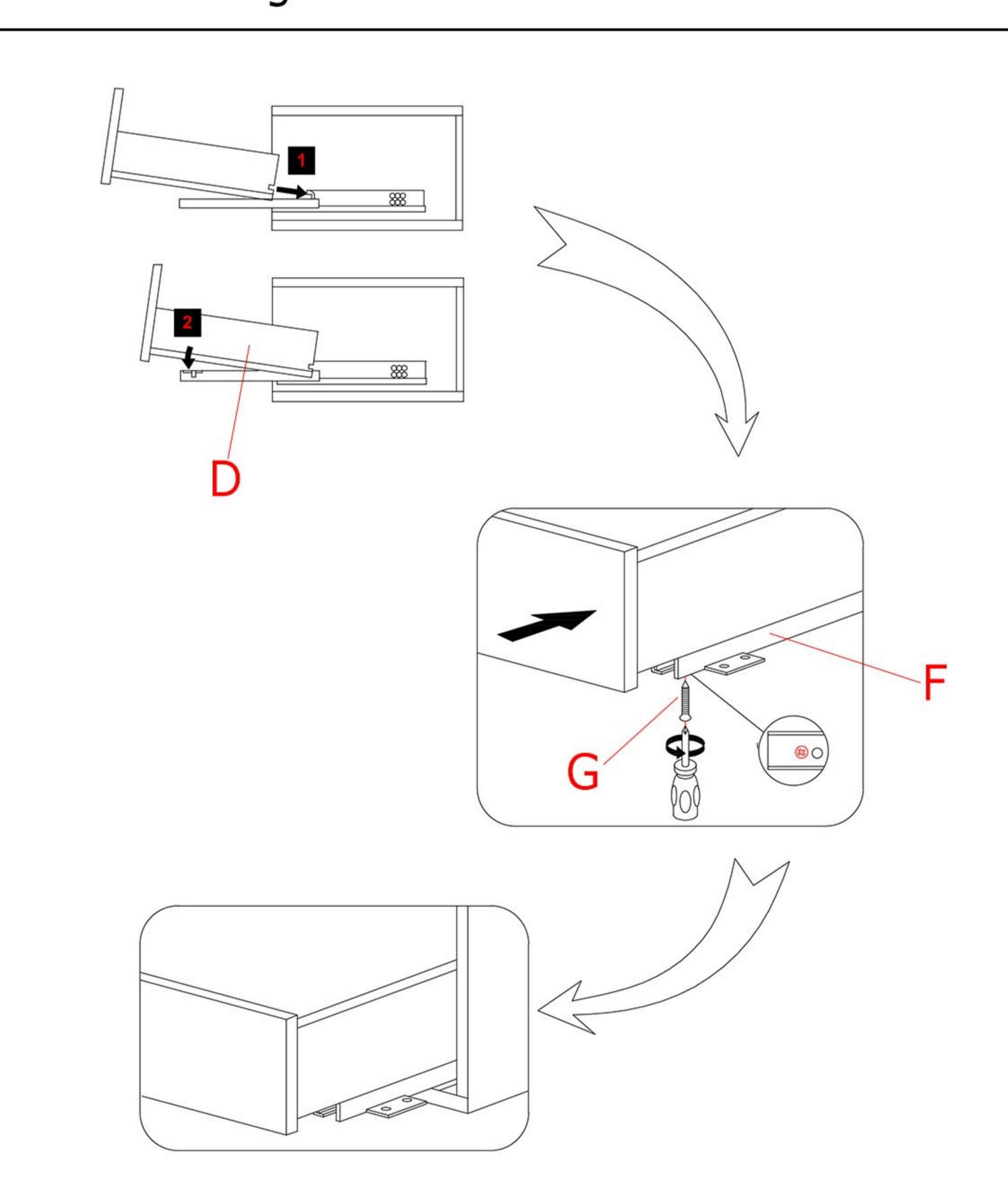
4. Screw on the self-tapping screws (G) to combine the drawer (D) with the slide rails (F).
