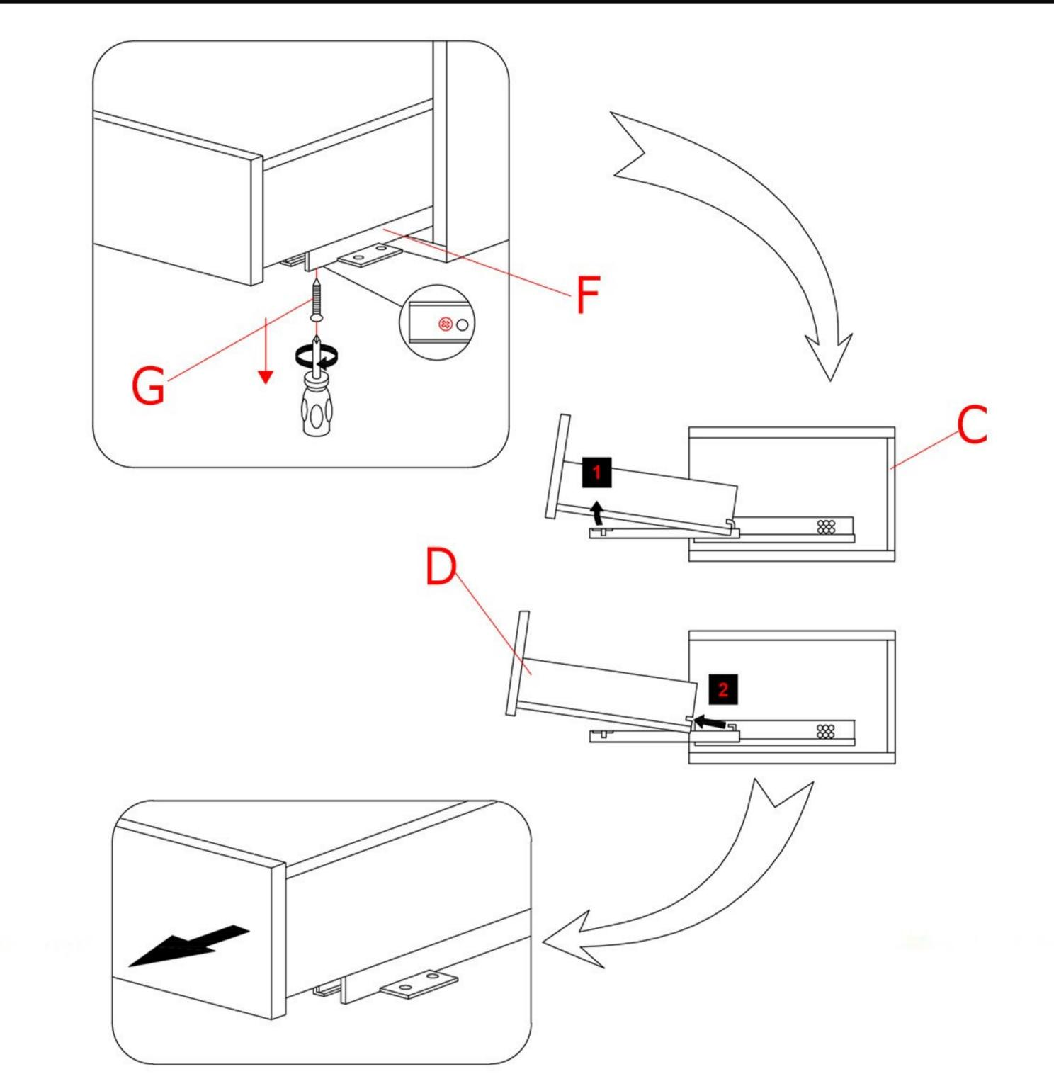
1. Unscrew the self-tapping screws (G) at the bottom of the drawer (D) and take out the drawer from the slide rails (F) inside the cabinet body (C).
